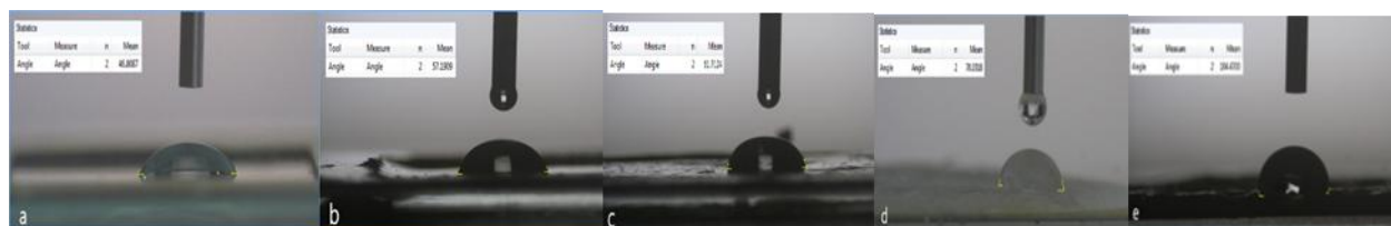
Figure 9 – Images captured by the contact angle measurement device for samples coated on glass slides are shown. As observed from the images, the contact angle increases with the epoxy coating, and further increases as the nanoparticle content in the epoxy matrix rises. a) bare glass slide, b) glass slide coated with epoxy, c) glass slide coated with a composite of epoxy matrix and amorphous nanoparticles, d) glass slide coated with a composite of epoxy matrix containing 30% GPTMS closed-ring functionalized nanoparticles, e) glass slide coated with a composite of epoxy matrix containing 30% GPTMS opened-ring functionalized nanoparticles.
